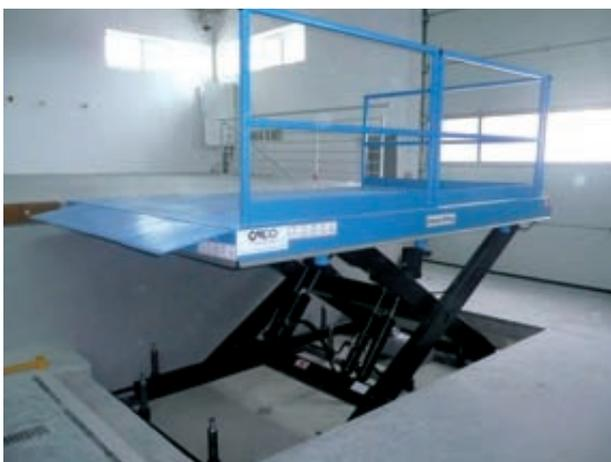
Loading processes lifting table with safety handrail and manual bridge plate
