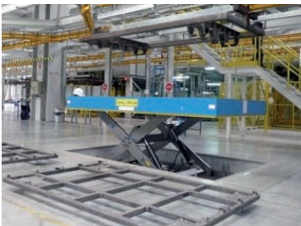
Industrial plants lifting table for a special application in a car factory
